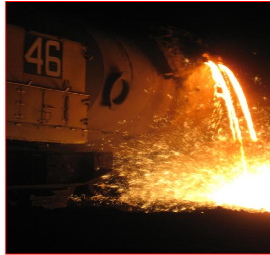
This picture shows the torpedo during wash out.
