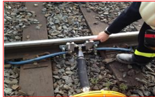
This picture shows the Rail Grease Unit.
